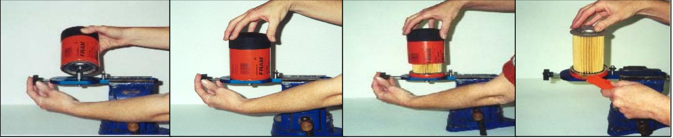
1. Place Oil Filter Cutter (OFC) in vise.
