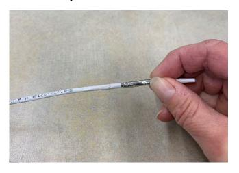
\* Using a razor blade score and crack jacket for strip length
