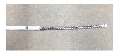
\* Use a small scissors to cut shield lengthwise
