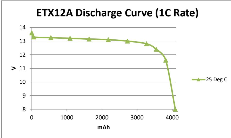
The graph below illustrate that usable Ah is nearly the same regardless of the discharge rate, with the voltage remaining above 11.5V for most of the discharge cycle.
