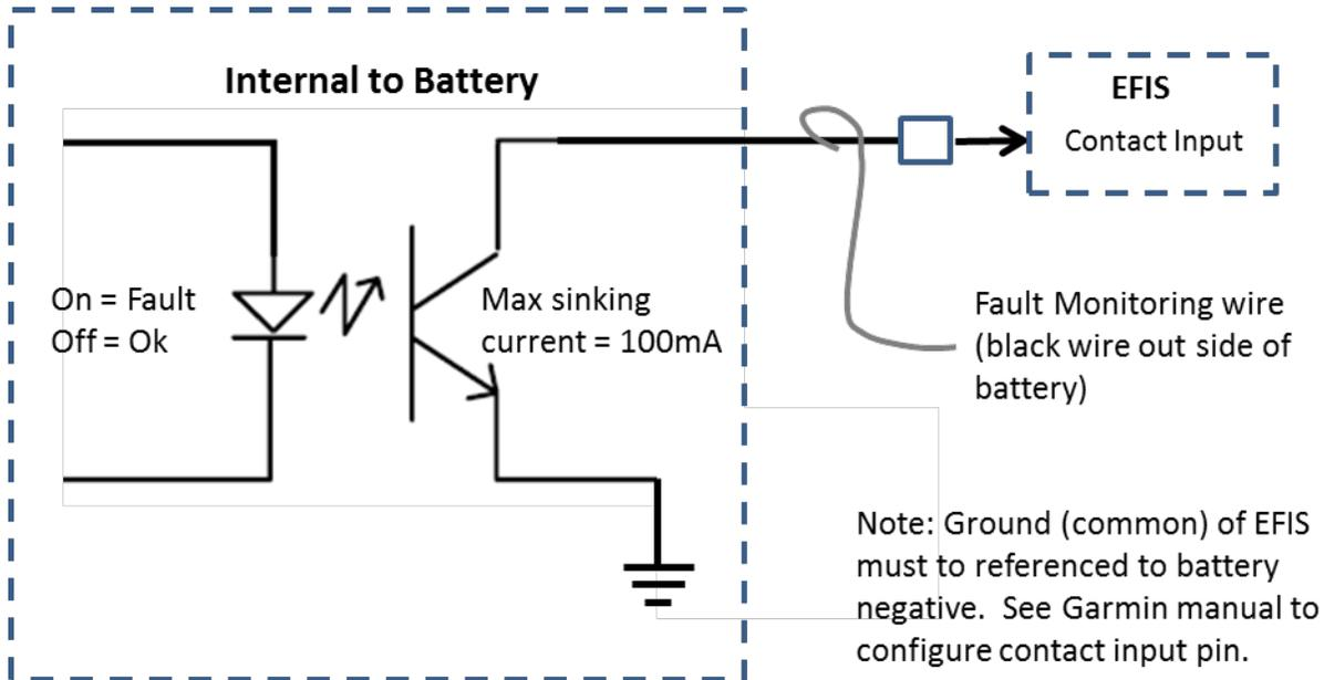
Configure the digital input (contact input) as “active low”, “user defined alert” type.
