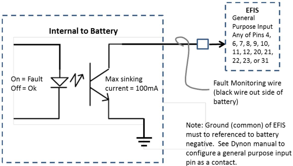
Configure the input as “active low”, “alarm” type. Note; when Dynon power is off the LED inside battery may be dimly lit (less than 120uA, too small to drain the battery).
