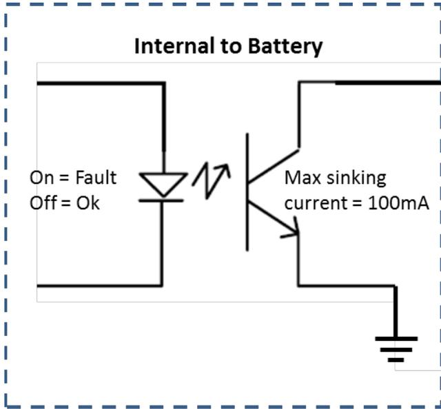
Setup Note: connect directly to an analog input (no external pull-up resistor needed).
