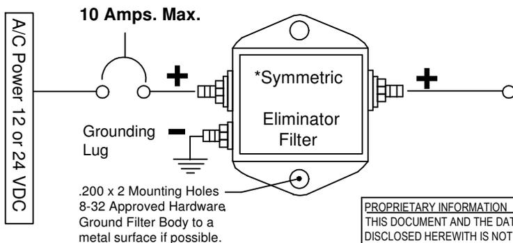
\*Symmetric : Power can be applied to either (+) terminal. Aircraft Electronics Effected by unwanted EMI-RFI Noise.
