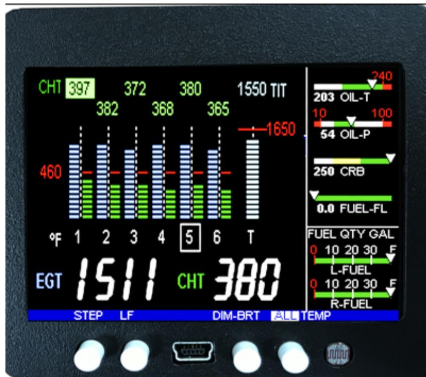
**EDM-350 system mounts in a 3.125 inch diameter instrument panel hole.**
