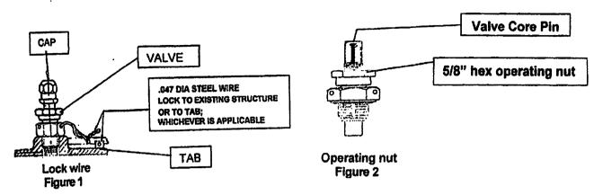
Never exceed pressure rating of the valve. This valve is rated for 3,000 PSI. All component parts used in the system to charge the valve must also be rated to be able to withstand the rated pressure or working pressure of the valve.
