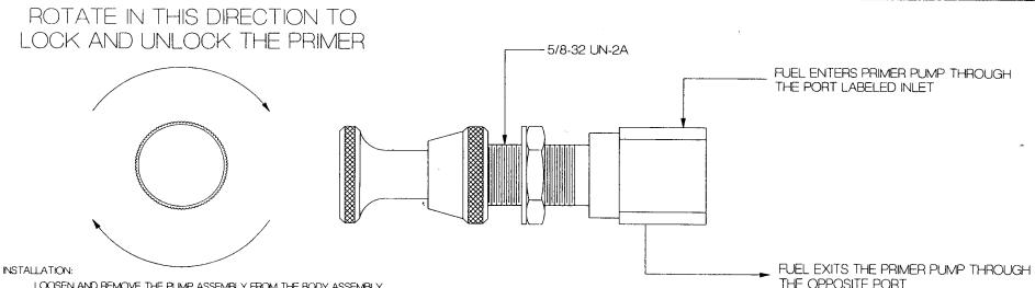
LOOSEN AND REMOVE THE PUMP ASSEMBLY FROM THE BODY ASSEMBLY BY UNSCREWING THE BEZEL NUT IN A COUNTER-CLOCKWISE DIRECTION. INSERT THE THREADED DIAMETER ON THE BODY ASSEMBLY THROUGH AN
